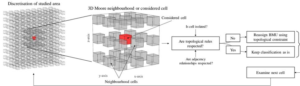
**Figure 2.** Summary of topological filtering used during post-regularisation.
