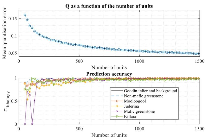
**Figure 8.** (a) Elbow curve of the quantization error for the determination of the optimum number of neurons (or units) in SOM and (b) Prediction accuracy for the different lithologies present in the training and validation datasets.
