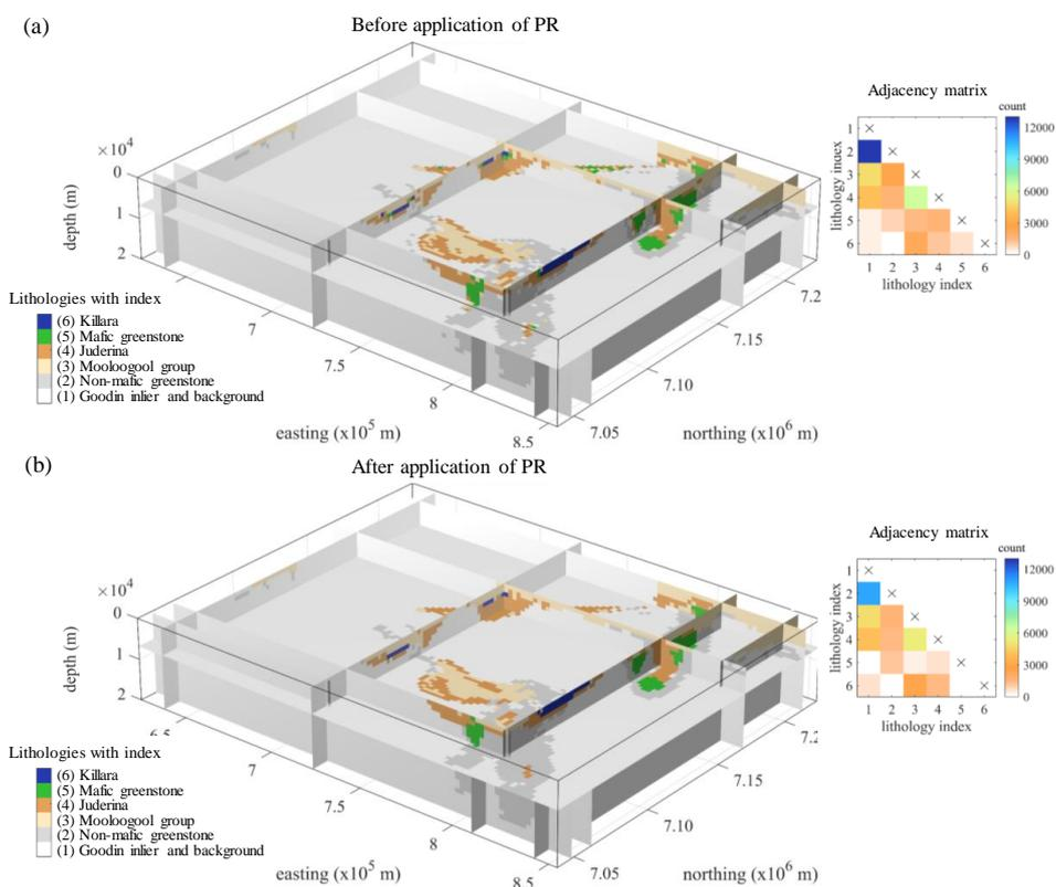
**Figure 9.** Recovered lithologies before post-regularisation (a) and after (b) next to the corresponding adjacency matrix (right hand side). The indices used to designate lithologies are indicated in the legend of the volume (left hand side).
