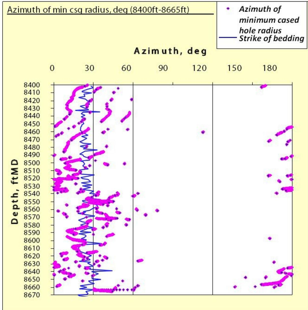
Figure 1. Reproduction of de Pater and Baisch fig 31, for Preese Hall-1, showing well log azimuths (lilac) and interpreted bedding strike from CMI imaging (blue).
