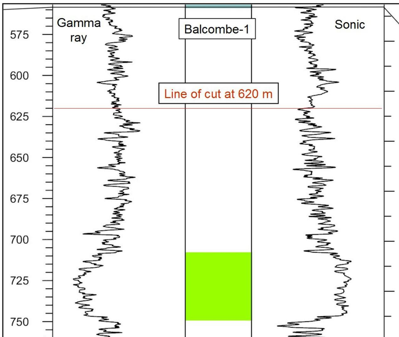
*Figure 3. Reproduction of detail of litholog (centre) and wireline logs from Andrews (2014). White on litholog is Kimmeridge Clay, green is the I-micrite. Depth on metres subsea. Red line shows where the cut has been made to match the logs to the Southwater-1 well (Fig. 4).*
