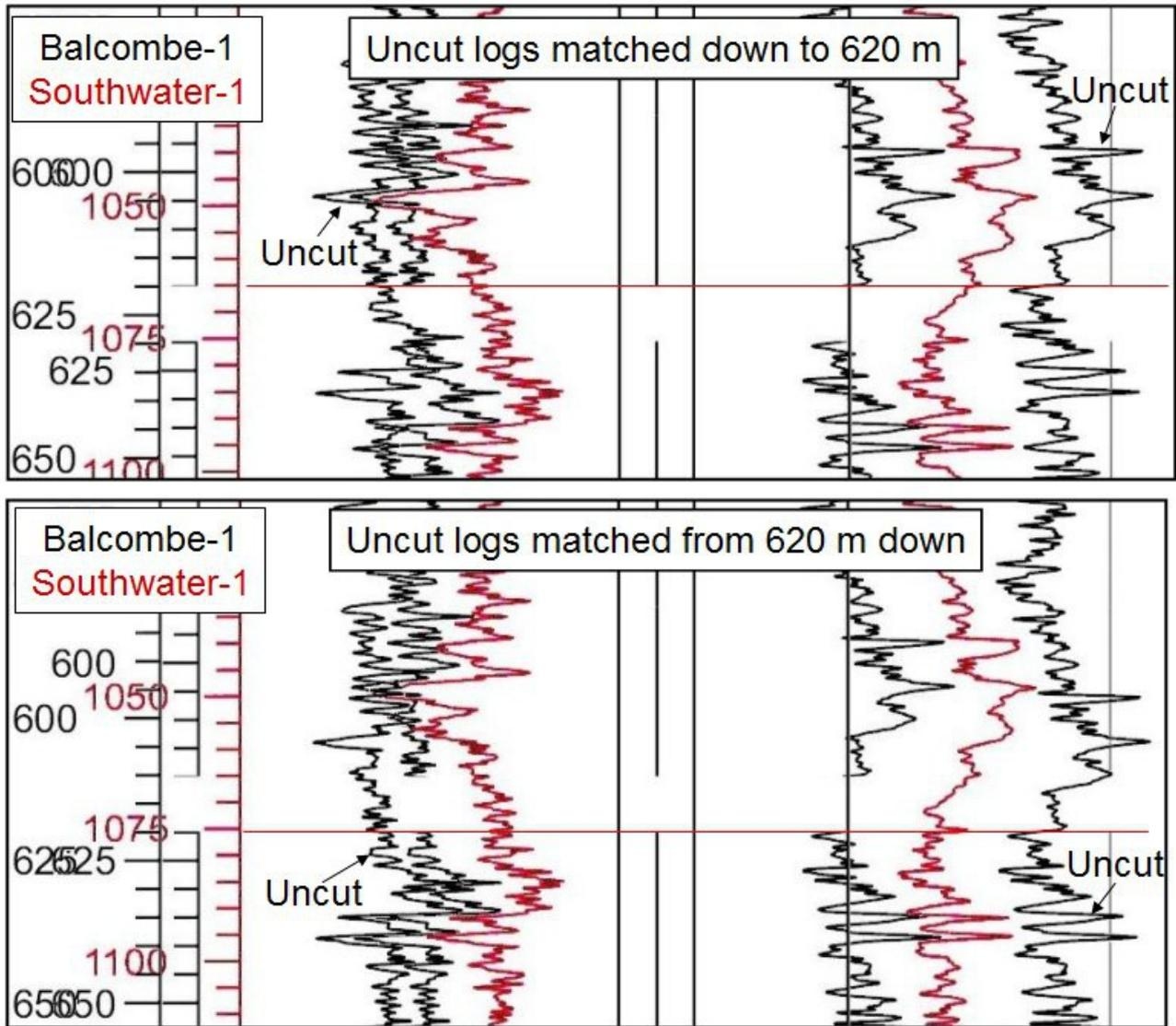
Figure 4. Detail from Smythe discussion paper figure 8A to demonstrate the process of matching up Balcombe-1 (logs in black), with its missing section, to Southwater-1, with its presumed complete section (logs in red).
