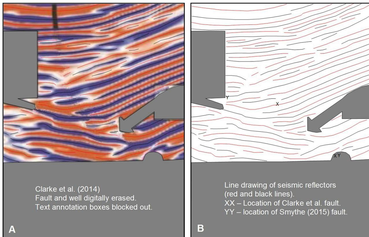
Figure 2. A. Clarke et al. (2014, fig. 4) sample of east-west 3D seismic through the Preese Hall-1 well. B. Line drawing of reflectors with alternative fault positions noted. The semicircle on the lowermost blocked-out area is the upper half of the hypocentral location.
