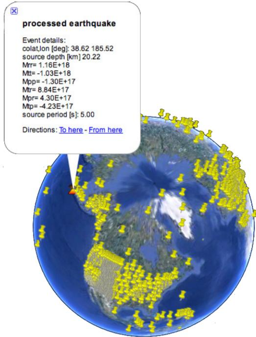
**Fig. 4.** A Google-Earth rendition of the source-receiver geometry used in an AxiSEM simulation. A generic output of the post-processing embedded within AxiSEM, this *kml*-file contains earthquake parameters (red dot), and actual seismogram images as links at the station locations (yellow pins).
