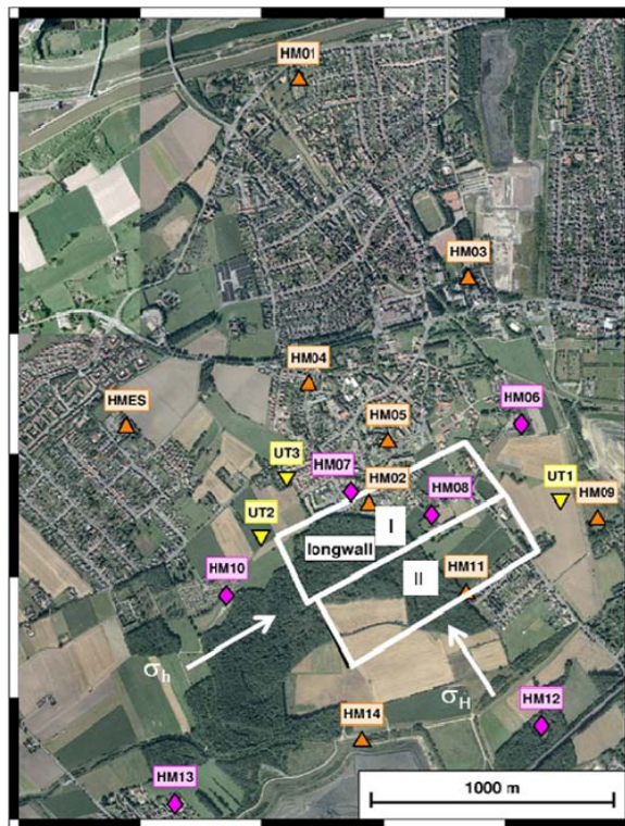
Fig. 2. Aerial view of longwalls, orientation of horizontal stresses and stations (Mine A).
